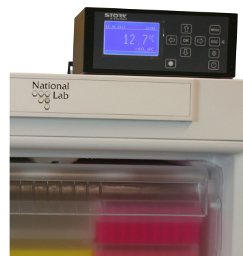
Temperature controller with graphic display and data logger
